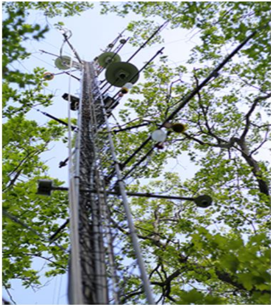
The AmeriFlux eddy covariance tower is used to measure gas and energy exchange between the ecosystem and atmosphere at the Harvard Forest in Massachusetts. Credit: Rick Wehr
