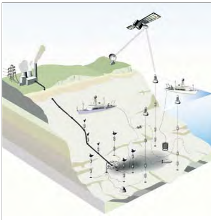
Figure 6.22 Schematic of possible approaches for monitoring the injection of CO 2 into the deep ocean via a pipeline. The grey region represents a plume of high CO 2 /low pH water extending from the end of the pipeline. Two sets of chemical, biological and current sensors and two underwater cameras are shown at the end of the pipeline. An array of moored sensors to monitor the direction and magnitude of the resulting plume can be seen around the pipe and are also located along the pipeline to monitor for possible leaks. A shore-based facility provides power to the sensors and for obtaining real-time data and an autonomous underwater vehicle maps the near-field distribution of the plume. A towed undulating pumping system monitors at distances of more than a few kilometres from the injection site. The towed system could provide much greater measurement accuracy and precision, but would also be able to provide measurements over large areas in a relatively short period of time. Moored systems are used to monitor the plume between mapping cruises. These moorings have surface buoys and make daily transmissions back to the monitoring facility via satellite. The very far-field distributions are monitored with hydrographic section cruises conducted every 2–5 years using standard discrete sampling approaches. These approaches provide the accuracy and precision required to detect the small CO 2 signals that add to background variations.
