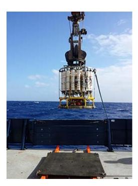
The rosette water sampler is used for repeat hydrography cruises like those sponsored by the Global Ocean Ship-Based Hydrographic Investigations Program (GO-SHIP) and ocean time series measurements. Credit: Leticia
