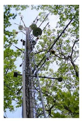
The AmeriFlux eddy covariance tower is used to measure gas and energy exchange between the ecosystem and atmosphere at the Harvard Forest in Massachusetts.
